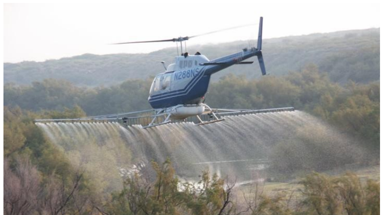
Use of helicopters to apply herbicide provides the convenience of aerial application with the added benefits of allowing precision application, virtually eliminating chemical drift, and allowing the landowner to selectively treat very specific areas.
