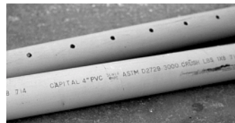
Figure 3. The drains consist of solid-wall pipe and perforated-wall pipe.
