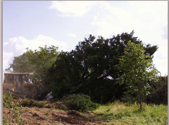
Dozers are effective at removing undesirable vegetation. This operator is selectively removing cedar only while retaining beneficial species. Photo © Clayton Wolf, TPWD
