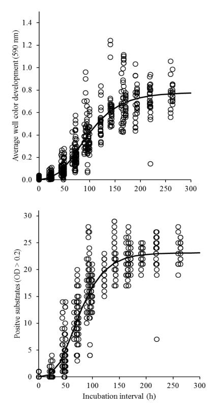
FIGURE 1.—Average well color development values and numbers of positive Biolog<sup>™</sup> EcoPlate substrates at increasing incubation intervals for 28 water samples from Possum Kingdom State Fish Hatchery ponds in November 2009 - May 2010. The solid trend line is a bestfit sigmoid curve.
