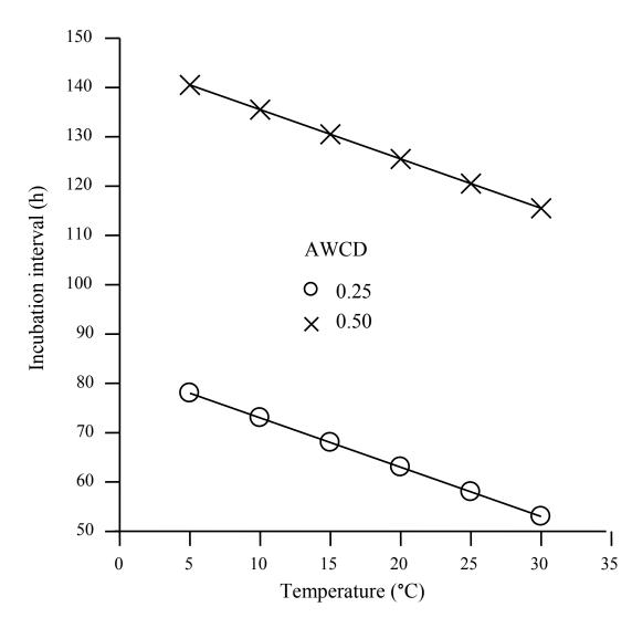
FIGURE 3.—Relationship between pond water sample temperature (°C) and incubation interval (h) required to achieve an average well color development (AWCD) value of 0.25 or 0.50. The linear regression equation of AWCD = -0.082 + 0.004\*hours + 0.004\* temperature was derived from 28 water samples from Possum Kingdom State Fish Hatchery ponds in November 2009 – May 2010 incubated on Biolog <sup>TM</sup> EcoPlates.
